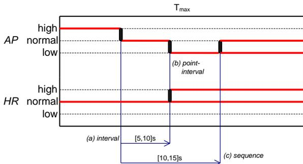
Figure 2: An ATC with temporal constraints defined between some nodes on the courses of the parameters AP (arterial blood pressure) and HR (heart rate).
