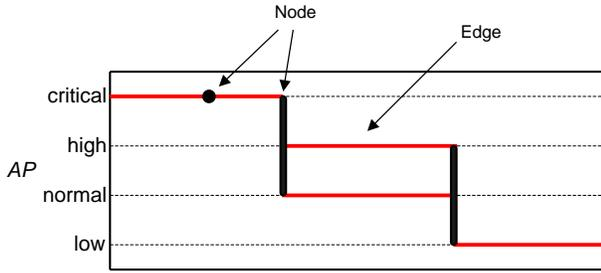
Figure 1: Edges and nodes in a parameter sequence in an ATC. Nodes can be defined at arbitrary positions on edges. They denote events expressing value changes and value persistence.
