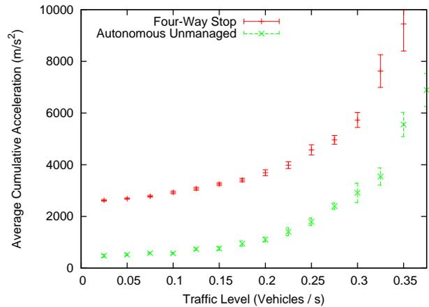
**Figure 3: A comparison of average acceleration of the four-way stop and our unmanaged mechanism. The x-axis represents the traffic level, expressed in vehicles per second. The y-axis represents the average of each vehicle’s cumulative acceleration, in meters per second per second.**
